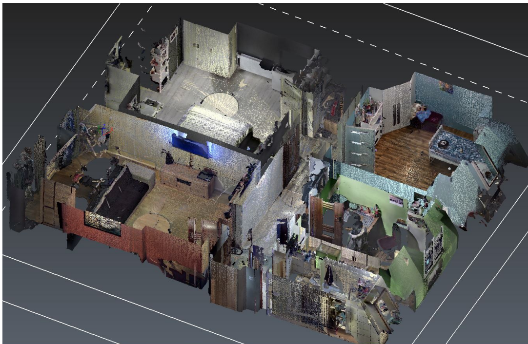
Figure 21 Point cloud generated for the demonstrated apartment
