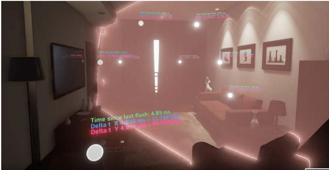
**Figure 12: Illustration of HTC vives positioning system with IR-line lasers sweeping the room.**
