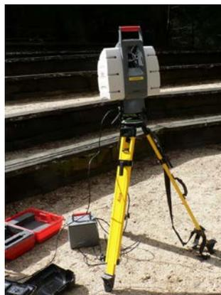
**Figure 6: 3D-laser scanning unit.**
