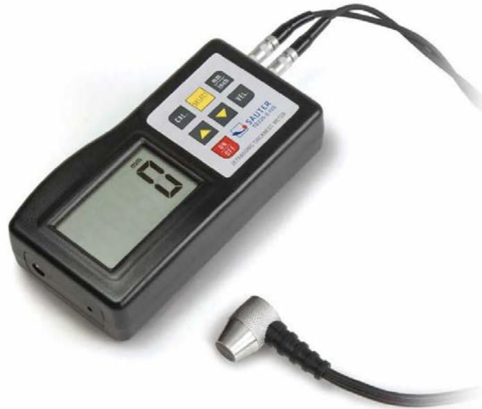
**Figure 9: Ultrasonic thickness gauge.**
