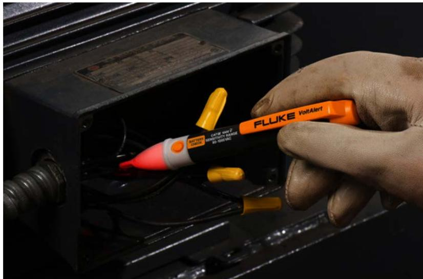
Figure 2: A contactless voltage detector. The read light at the tip shows that the cables are alive.
