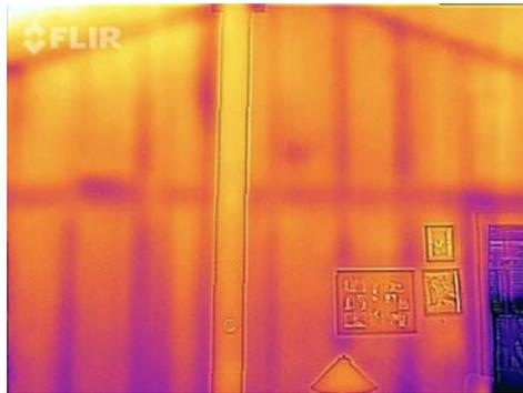
**Figure 3: Studs visible in the wall due to their heat conducting properties.**
